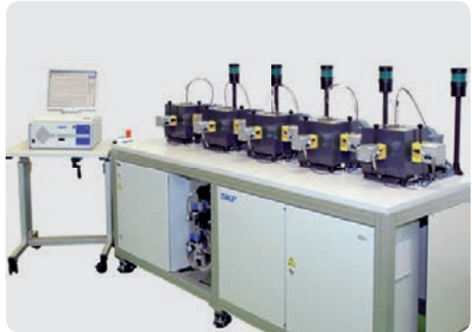
ROF+ grease test rig
