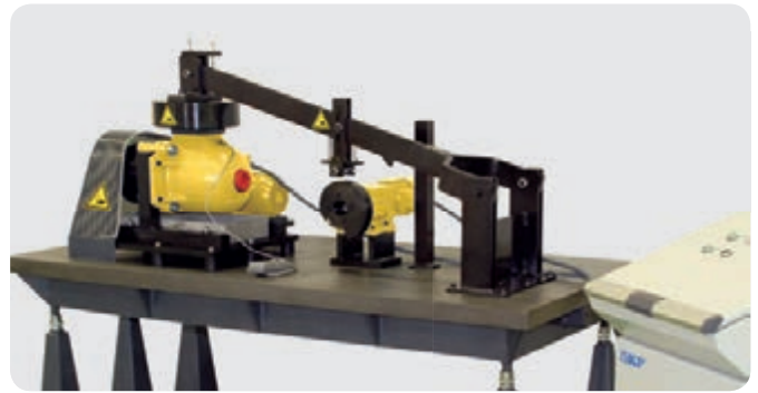
V2F grease test rig
